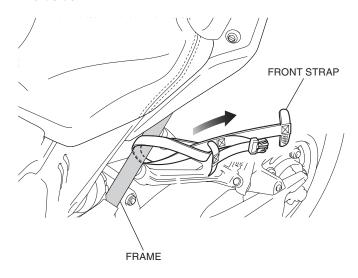
5. Route the front strap, and then secure the strap end as shown.
